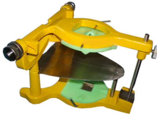
UNIVERSAL ARTICULATOR (YELLOW) JU-81-114 UNIVERSAL ARTICULATOR OPENING 125° WITH 4 MOUNTING PLATES - CONDYLAR INCLINATION FIXED AT 30°, INTERCONDYLAR DISTANCE AT 110MM, BENNET ANGLE FIXED AT 7°, DISTANCE BETWEEN MOUNTING PLATES 85 MM. SOLIDLY CONSTRUCTED OF METAL ALLOY CASTING. Available In Assorted Colors
